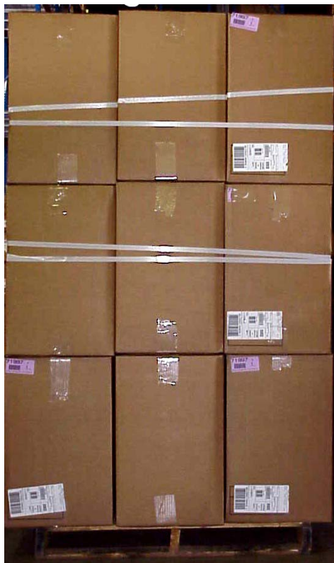
Non-conforming – single pallet height / product overhang / not shrink wrapped.
