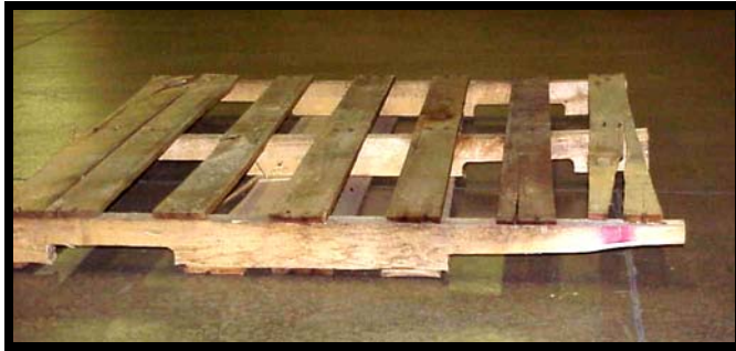
Non-conforming - broken pallet
