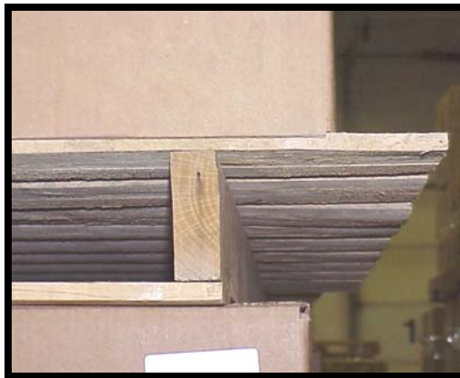
Non-conforming - deck board overhang
